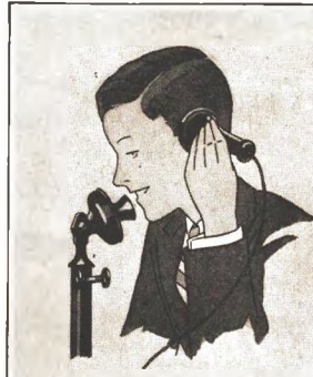
Speak directly into the transmitter with the lips close to but not against the mouthpiece.
